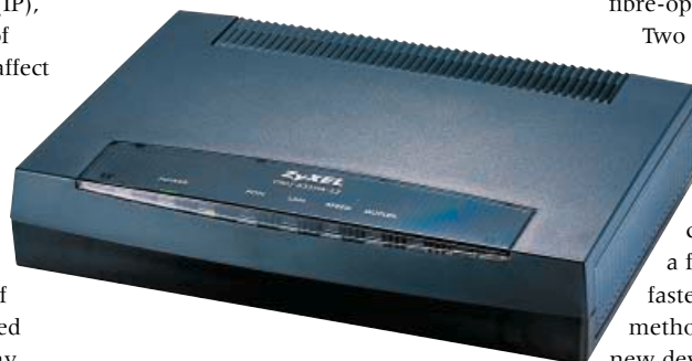
In a fibre network an Optical Network Terminal takes the place of the broadband modem we're used to
